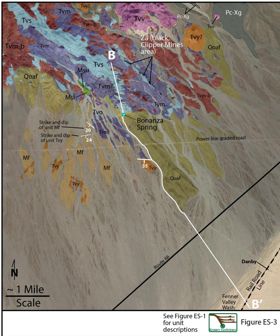
Figure ES-3 Geologic map showing Cross Section B-B' along Bonanza Wash
